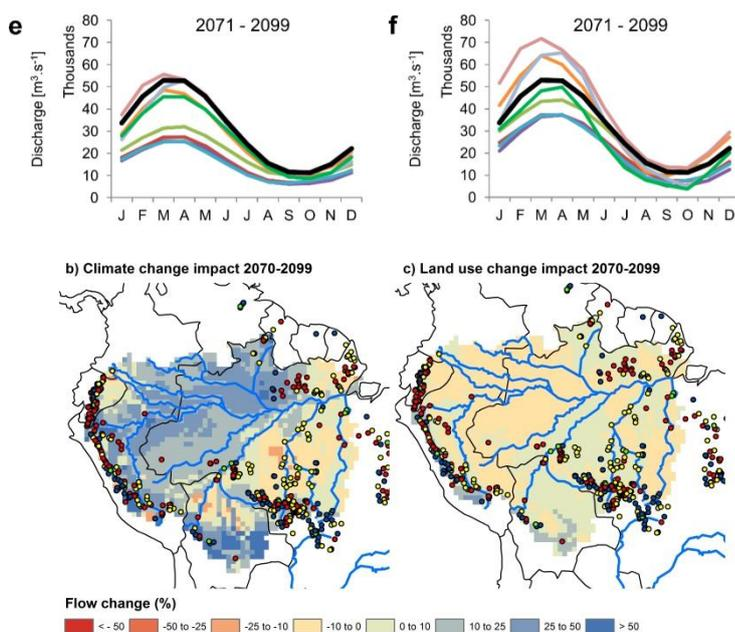
Figure 5 Simulated hydrographs of Rio Madeira (top, Brazilian model) and discharge (bottom, LPJml model), for climate change only (left) and including LUC (right).
